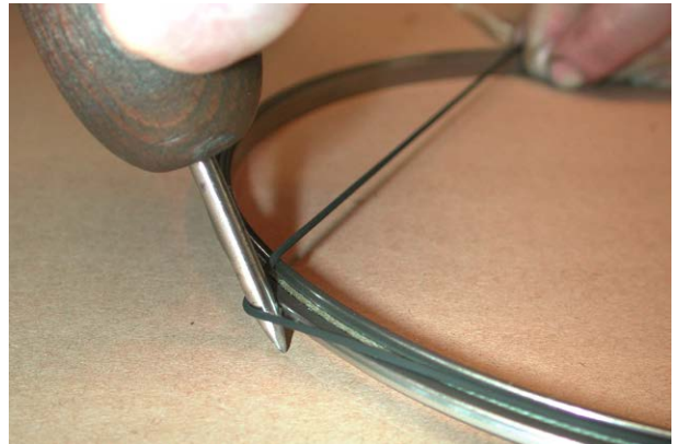
22. Detail view of the rubber seal installation.
