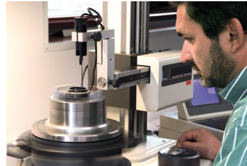
Inspection of Ring Concentricity by PROSINO S.r.l.
