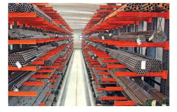
Prosino's flexibility is granted by a very well stocked storehouse with 100Cr6 steel tubes, in more than 100 sizes. Turning operations are carried out for small diameter rings and for high quantities using GILDEMEISTER multispindle mechanical lathes with bar capacity of 100 mm. Prosino autonomously manufactures shaped tools with modern EDM profiling machinery, granting a very low roughness level. This improves the production autonomy and flexibility.
